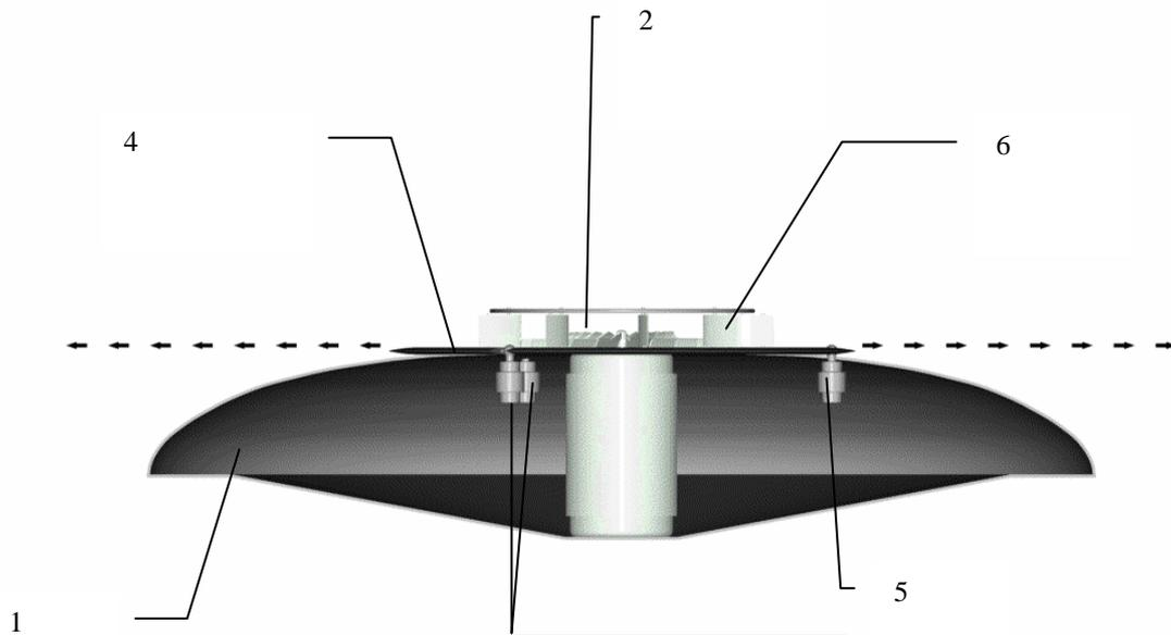
The lift and propulsion control mechanism is a circular aerofoil disposed around the motor torque cancellation and steering mechanism controlled by a number of linear actuators such that it can be moved uniformly up and down as illustrate or inclined.
