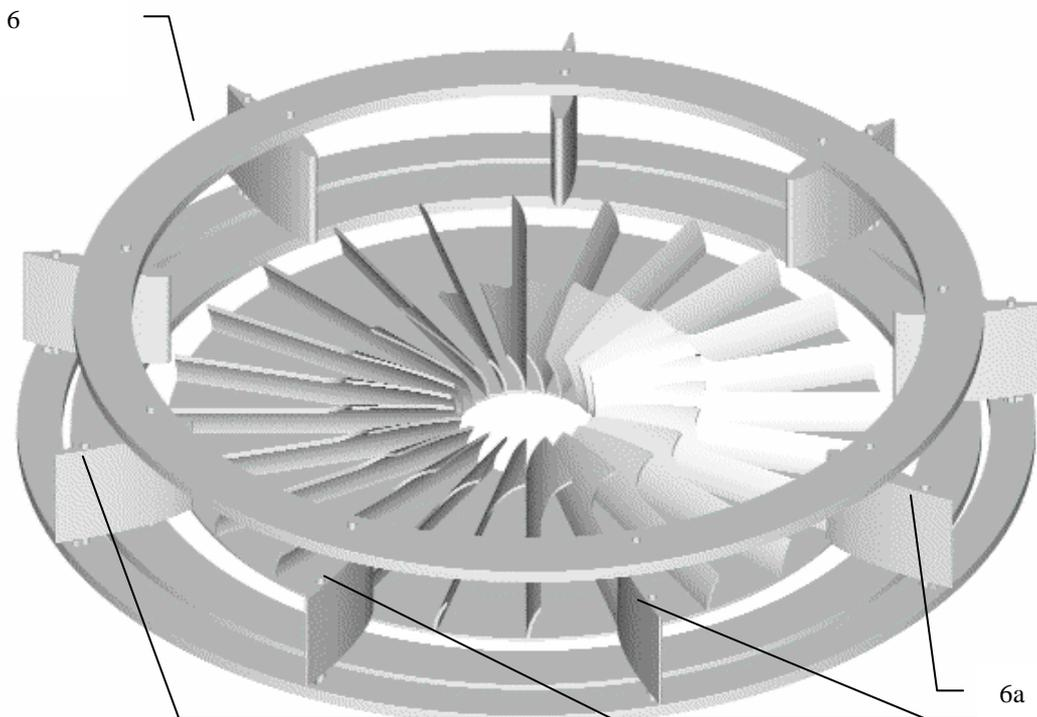
**Close up detail of the disk fan and motor torque cancellation and steering mechanism**
