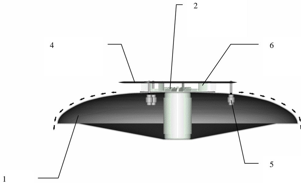
In the second illustration, the lift and horizontal propulsion control mechanism is uniformly raised such that the air stream from the disk fan is allowed to attach to the upper surface of the UAV and hence there is maximum lift imparted to the aircraft.
