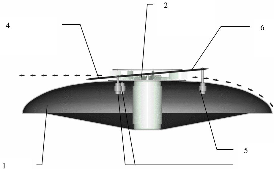
So in effect, lift and hence ascent and descent rate is controlled by the same passive mechanism as horizontal acceleration. I believe that this method of controlling the lift forces combined with directional control is unique to the Coanda design concept.
