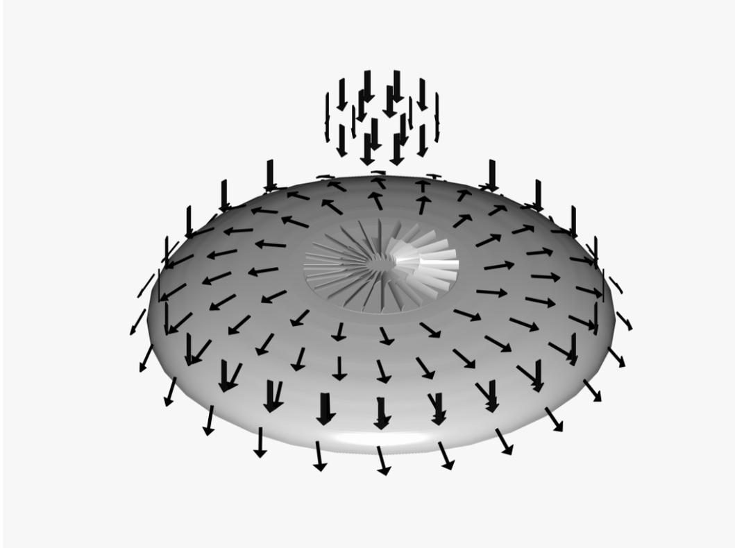
In this simplified illustration I have attempted to explain the lift mechanism. Air is drawn into the disk fan at the centre of the aircraft and a component of lift is developed by this action.
